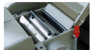
solid steel rotor with knife wedge mounting system massiv stålrotor montering kniv/knivkile
